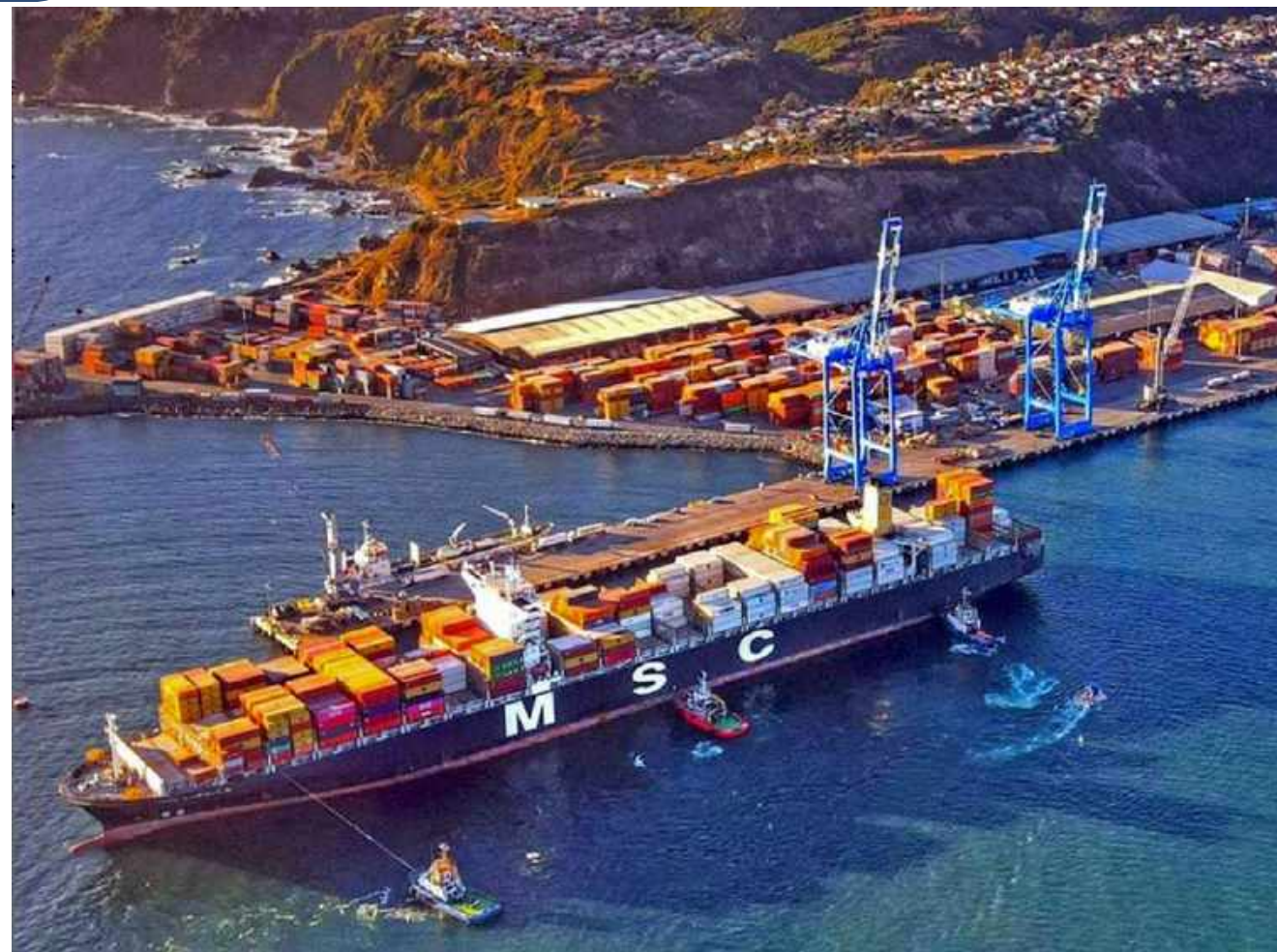
The MSC Capella in Puerto Talcahuano, Chile. The vessel – with a length of 366.45 m, a beam of 48.20 m and a capacity of 13 119 TEUs – became the largest ship ever to call in on San Vicente International Terminal (SVTI). Photo courtesy of www.msc.com/
