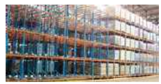
Narrow aisle pallet racking
