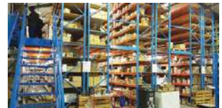
Rack supported multi pick levels
