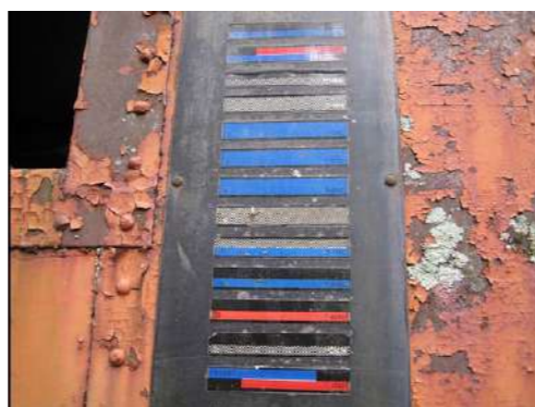
Left: Detail of a KarTrak code. This barcode is Start 8350199918 Stop 5. https://en.wikipedia.org
