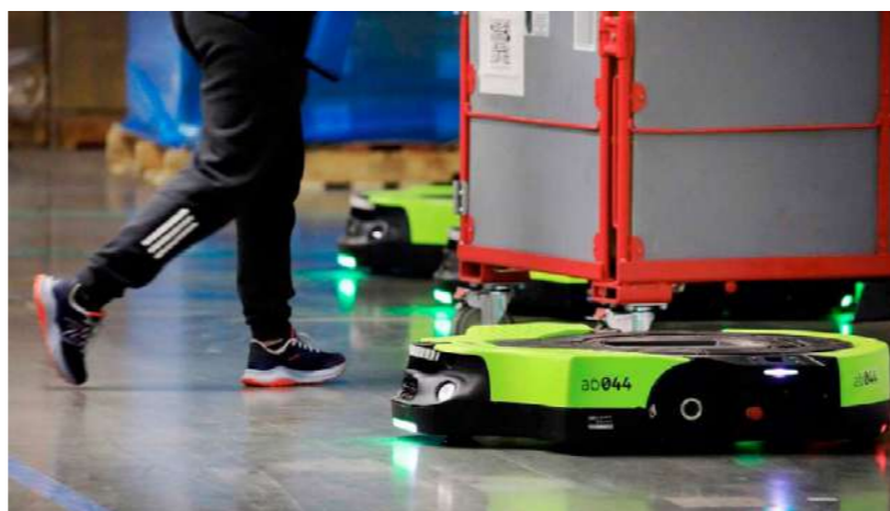
Proteus is Amazon's first fully autonomous mobile robot, meaning it can navigate freely throughout a site using sensors to detect and avoid objects in front of it. Other mobile robots, such as Titan and Hercules, are confined to areas where only authorised robotic specialists can enter, and read barcodes that are stickered to the floor as navigation coordinates. Proteus works in conjunction with Cardinal – a robotic arm that loads packages into carts – to move those carts from the outbound dock area of the fulfilment centre to the loading dock, where packages are loaded onto trucks. www.aboutamazon.com/news/operations/amazon-robotics
